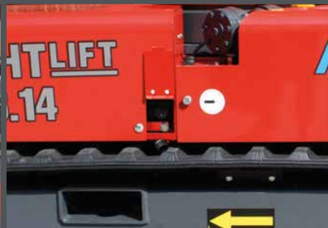
Auxiliary connector for external devices, telematics and fleet tracking.
