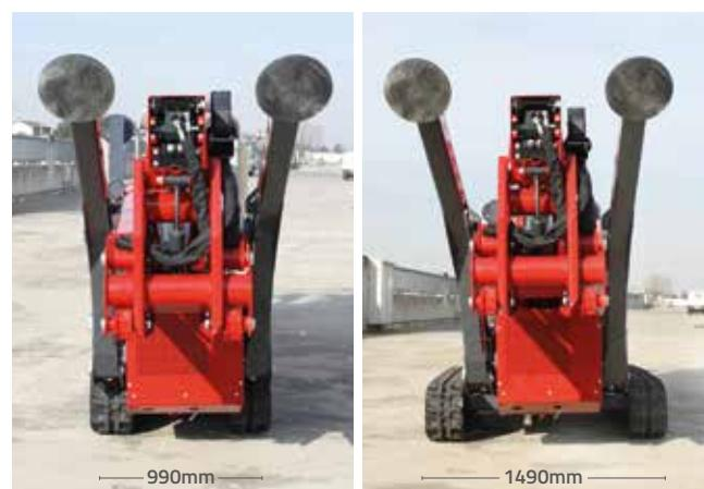
Incredible widening of the undercarriage, from 990mm allowing easy passage through narrow and cramped places, to 1490mm for an enhanced lateral stability.
