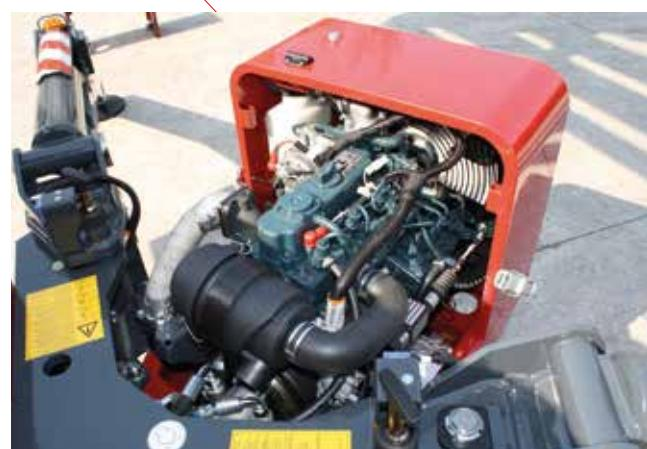
New Kubota Diesel D902 3 cylinder water cooled engine, meets the Tier 4 standards, with 40 litres capacity tank for an increased range.
