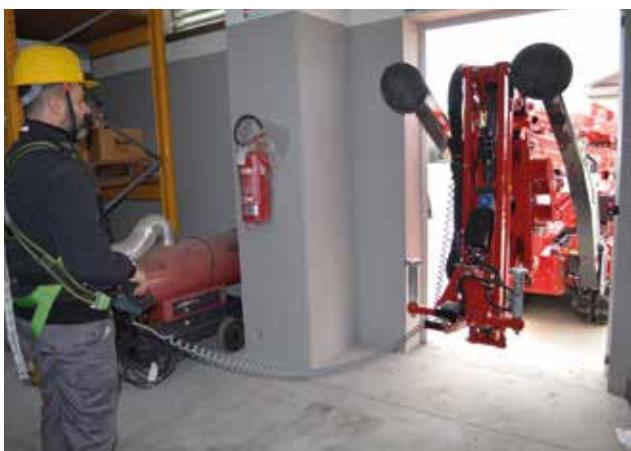
Height of the machine in transport configuration is less than 2m allowing easy passage through the doors.
