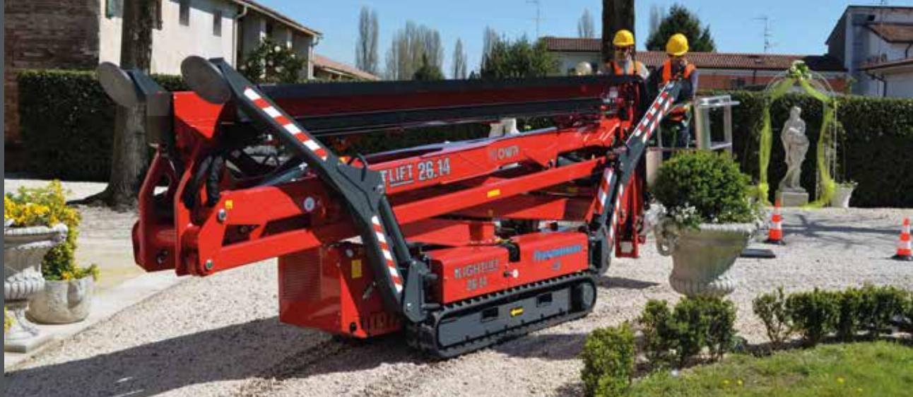
Lengthened undercarriage for greater stability, improved angle of attack (22°) and lowering of ground pressure during translation, equipped with Auto2Speed technology for maximum speed or torque depending on the working conditions.
