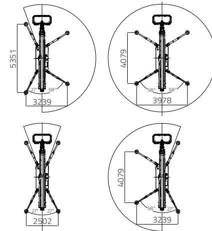
3 working stabilization areas. Working movements with optimized speeds.
