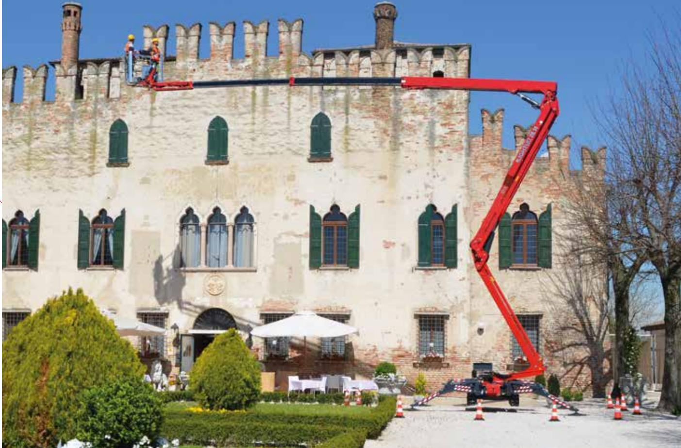
Articulated boom with double telescopic steel boom, in Domex® 700 with wall thickness from 3 to 5mm for max service life and stiffness.
